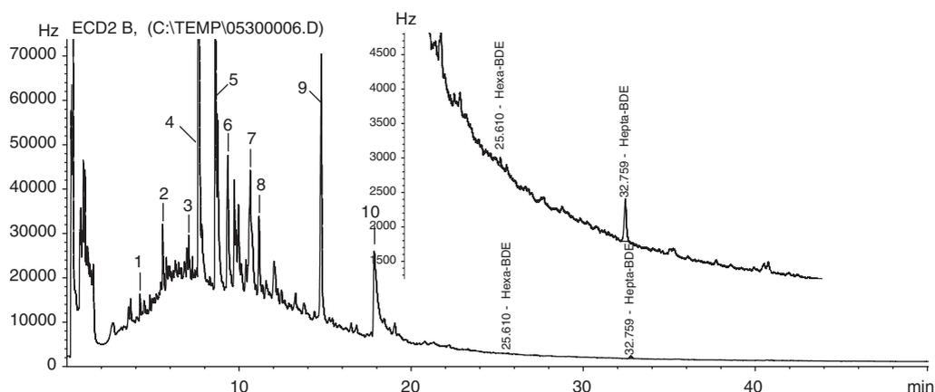
Figure 5. SPE-SFE-GC-ECD chromatogram of leachate water from Hårlöv Landfill, Kristianstad, Sweden, with 10 unidentified markers (1–10) and two identified PBDEs. Above the original baseline is the attenuated chromatogram to illustrate that the elution region for higher PBDEs is relatively free from interference. The concentrations of hexa-BDE (PBDE 153) and hepta-BDE (PBDE 183) are ca. 15 and 190  $\mu\text{g mL}^{-1}$ , respectively.
