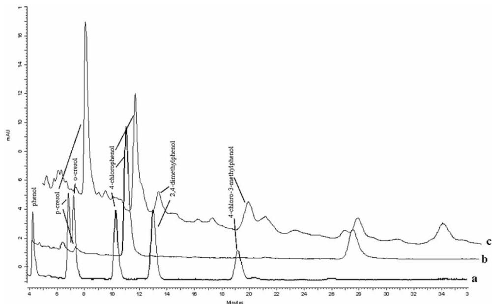
Figure 3. Three overlaid SLM-HPLC chromatograms at 280 nm, containing phenolic markers. Retention time and absorbance is offset for easier visualisation: (a) 50 ng mL<sup>-1</sup> standard, (b) leachate sample after ozone treatment from the pilot plant, and (c) raw leachate water Härlöv waste deposit, Kristianstad, Sweden.
