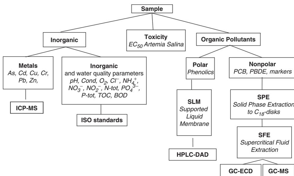
Figure 2. LAQUA-protocol: an analytical strategy for characterization of leachate and evaluation of the efficiency of different treatment procedures.
