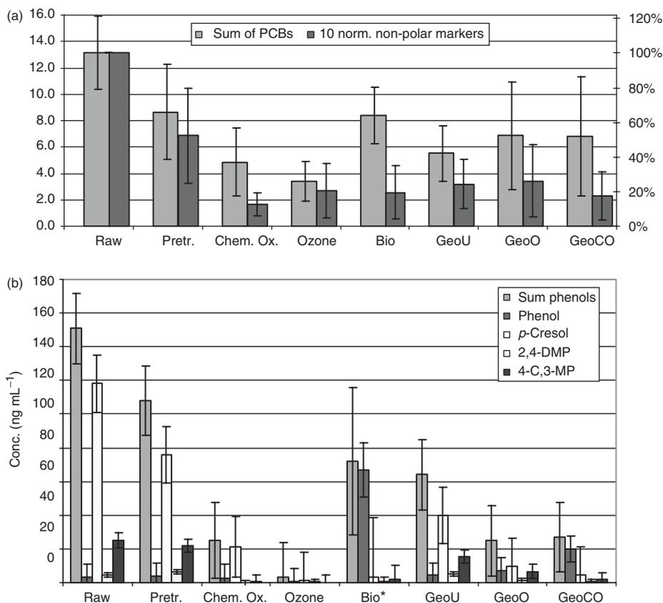
Figure 6. Treatment efficiency with respect to marker substances in different steps of the studied pilot plant. (a) Sum of PCBs (left) and of 10 unidentified non-polar organic compounds (right), normalised according to the text. (b) Results for sum of phenols, and for four major identified phenols. Error bars show the 95% confidence intervals for the average ( $n=8$  except for Bio\* where  $n=2$ ), of samples, obtained from time-integrated sampling at different dates.
