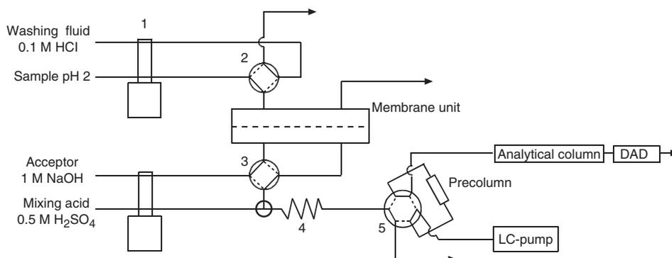
Figure 1. Schematic picture of the automated SLM extraction system; for details see text.
