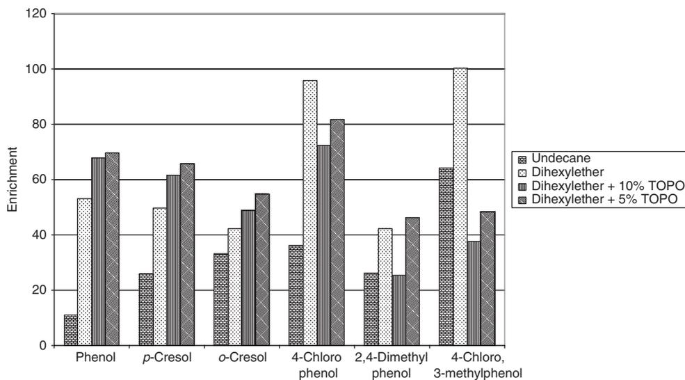
Figure 4. Enrichment factors for different membrane fluids for the investigated phenols, after 30 min extraction at  $1 \text{ mL min}^{-1}$ .
